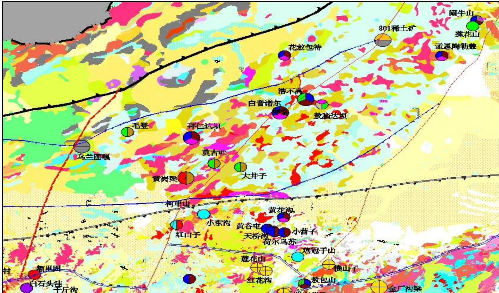
Late Paleozoic continental margin accretion belt and superposed by the Yanshanian magmatic belt. The Permian marine facies intermediate-mafic volcanic rock is developed, and it is favourable area for the marine facies volcanic Cu polymetallic deposit and Mesozoic porphyry W-Cu-Sn-Mo deposit.
