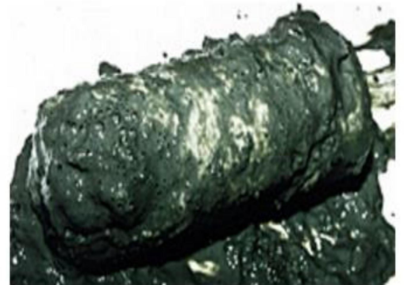
Concentrated gas hydrate (white material) covered with mud. This core was obtained on the Blake Ridge during Ocean Drilling Program Leg 164. Click image for larger view.
