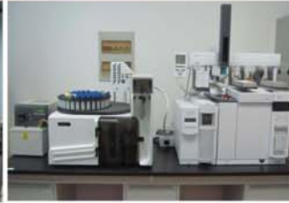
气相色谱-质谱联用仪 Gas Chromatography - Mass Spectrometry
