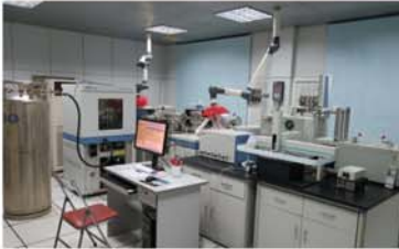
MAT253稳定同位素质谱仪 MAT253 Stable Isotope Ratio Mass Spectrometry
