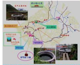
利用高位表层岩溶泉采取蓄—引技术开发利用，兴建地间水柜，建立了峰丛岩溶区立体生态农业模式 Using storage-with-diversion to develop high-level epikarst spring with water tank constructed to establish a comprehensive ecological mode for peak-cluster area.
